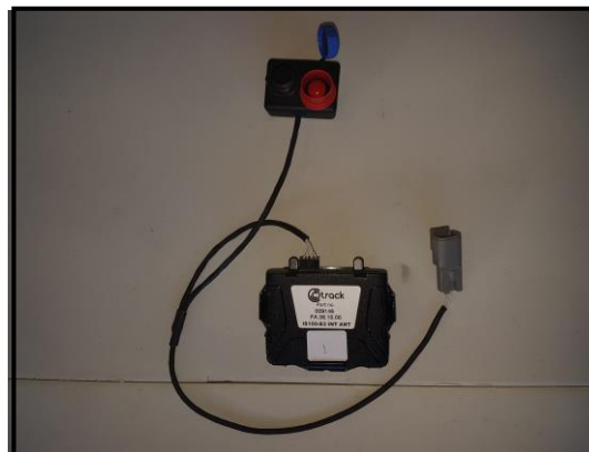
Panic Button Assembly & Ctrack Unit
