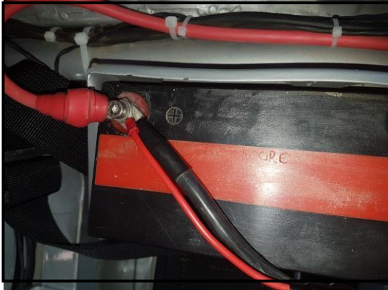
Permanent Power & Earth Connections
