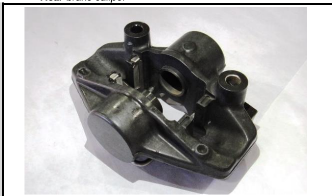
K4-6) Support d'étrier de frein arrière Rear brake caliper support
