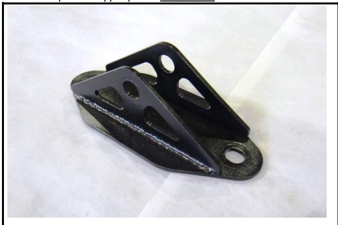
Typical joint of the rear axle version 2 with spherical bearing
