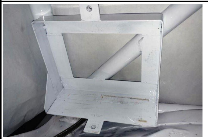
Battery bracket – dismounted
