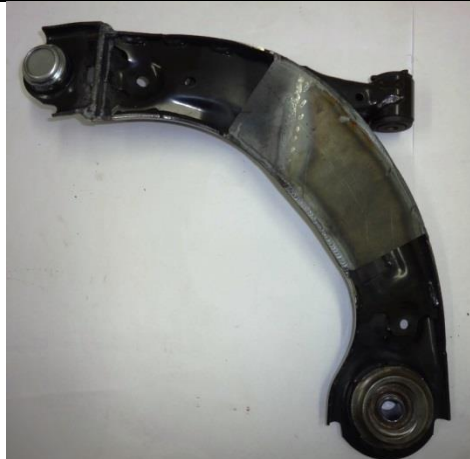
G5-2) Triangle/bras complet – déposé Complete wishbone/arm – dismounted reinforced ,lower
