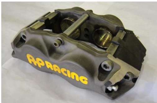
J4-5) Support d'étrier de frein avant Front brake caliper support
