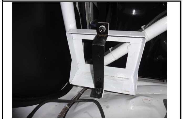
Battery bracket – mounted
