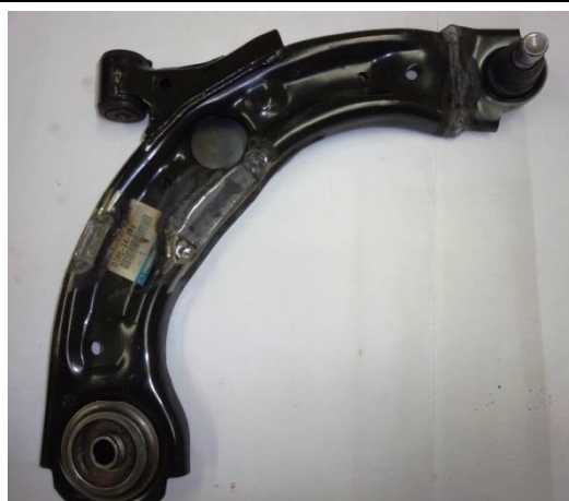
G5-2) Triangle/bras complet – déposé Complete wishbone/arm – dismounted reinforced ,upper
