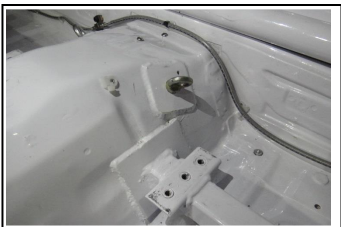
Seat belt fixations inner
