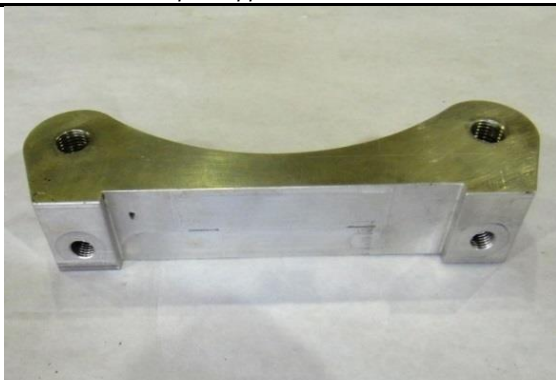
J4-5) Support d'étrier de frein avant Front brake caliper support
