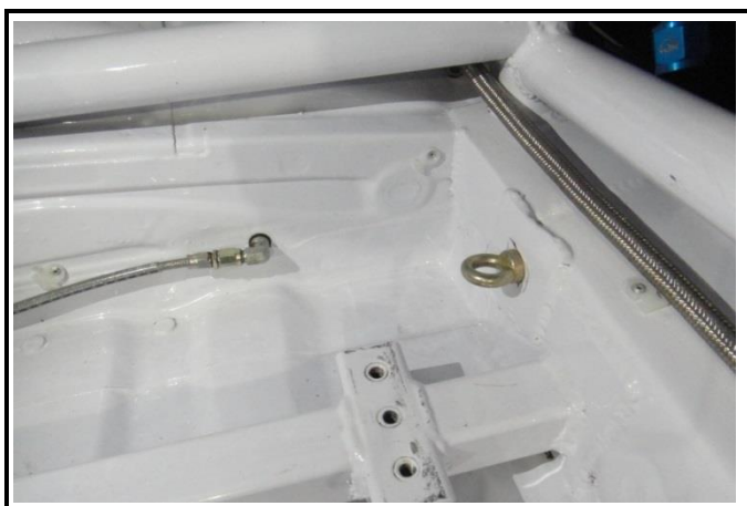
Seat belt fixations outer
