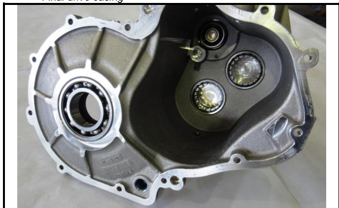
F4-1) Carter de couple final Final drive casing
