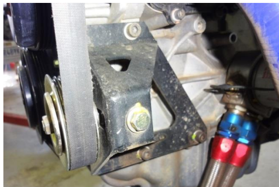
L3-3) Suppression du compresseur de climatisation - installation Removal of air conditioning compressor - installation
