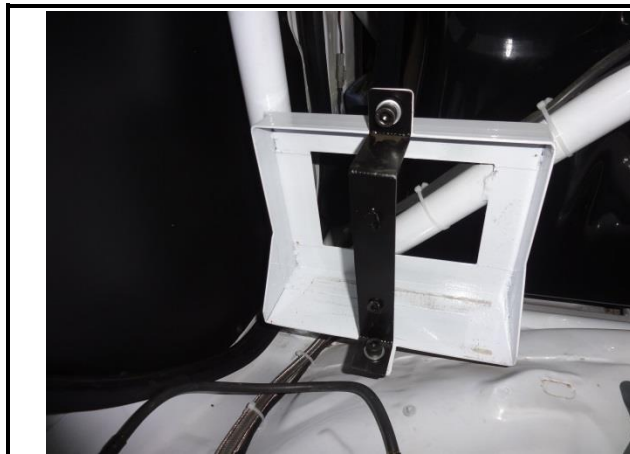
Battery bracket – mounted
