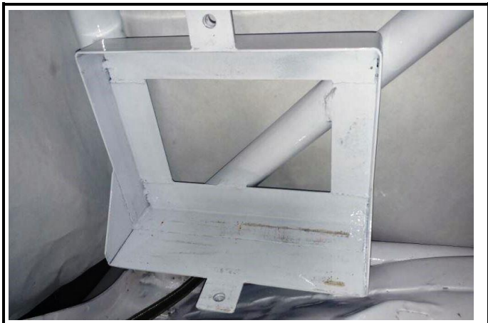
Battery bracket – dismounted
