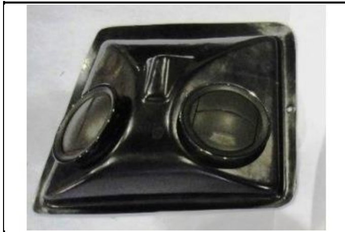
M1-2 Roof vent, inner
