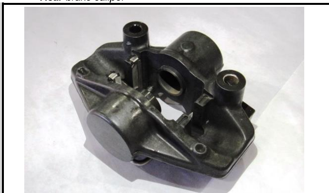
K4-6) Support d'étrier de frein arrière Rear brake caliper support
