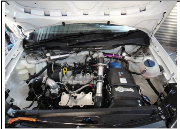
PHOTO 9: Engine bay and turbo air pipe lay-out
