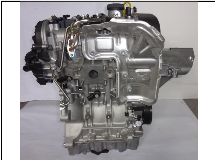
PHOTO 3: Engine exhaust side without turbocharger
