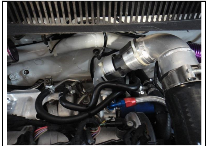
PHOTO 10: Turbocharger exit to intercooler
