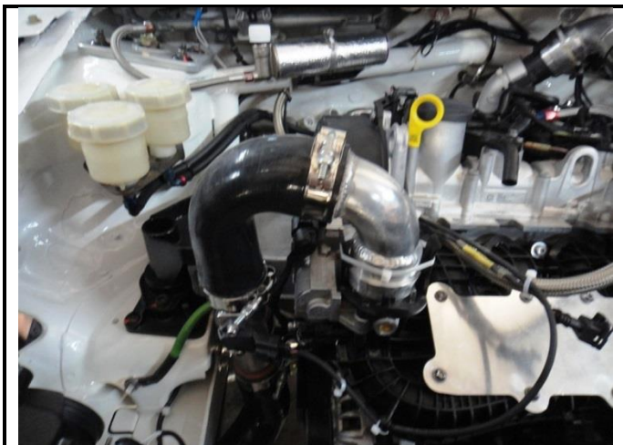
PHOTO 11: Intercooler to throttle body
