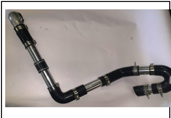
PHOTO 15: Turbo to intercooler pipe
