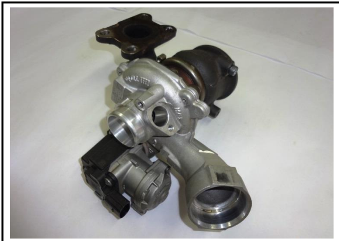
PHOTO 5: Turbocharger compressor
