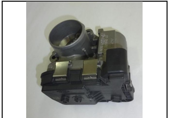
PHOTO 6: Throttle body intercooler side
