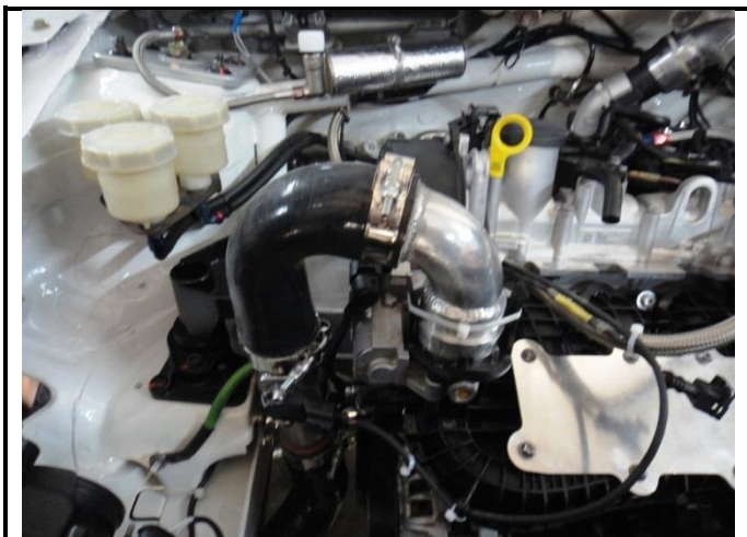
PHOTO 11: Intercooler to throttle body
