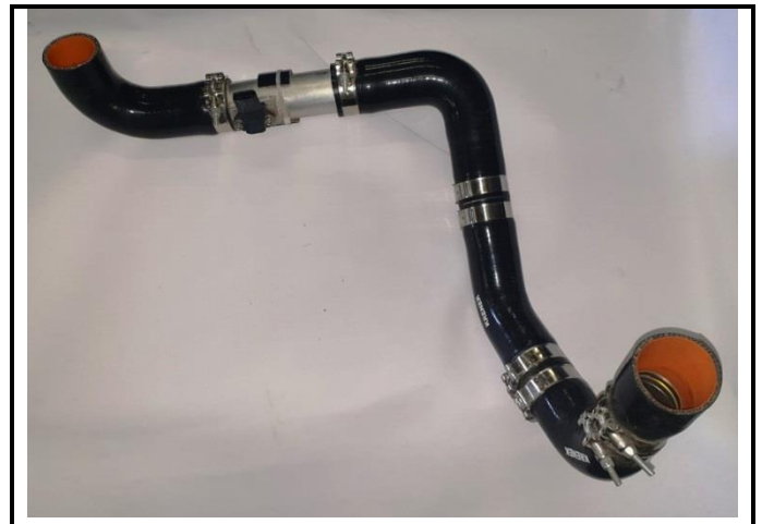
PHOTO 16: Intercooler to inlet manifold pipe with air temp sensor
