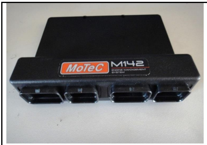
PHOTO 17: Motec M142 ECU dismantled
