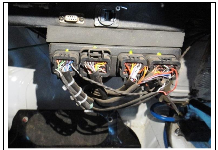
PHOTO 18: Motec M142 ECU mounted
