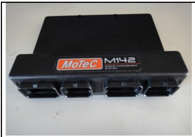
PHOTO 17: Motec M142 ECU dismounted
