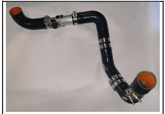
PHOTO 16: Intercooler to inlet manifold air pipe
