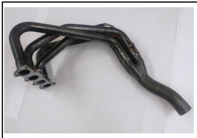
PHOTO2: 328 Exhaust manifold type 3.
