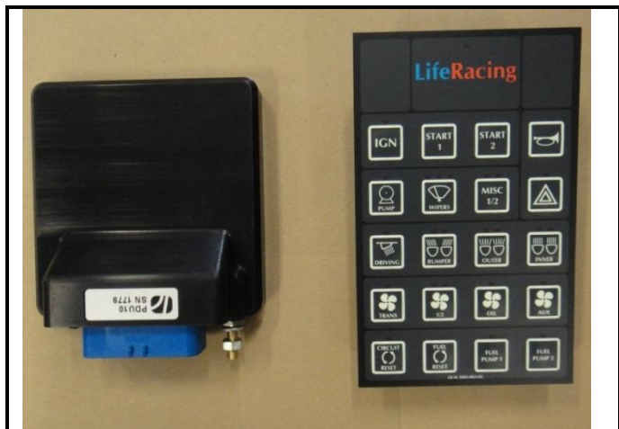
PHOTO 1: 324, Power Distribution Unit.
