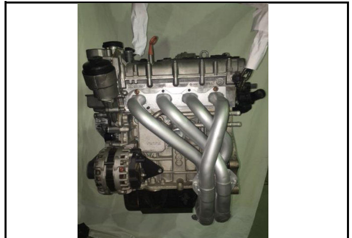
PHOTO 2: VW BAG 1.6 d.i, Exhaust side.
