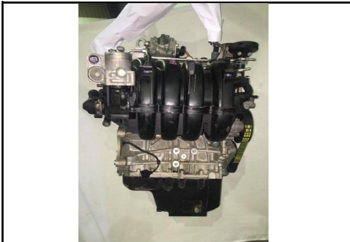
PHOTO 1: VW BAG 1.6 d.i, Inlet side.
