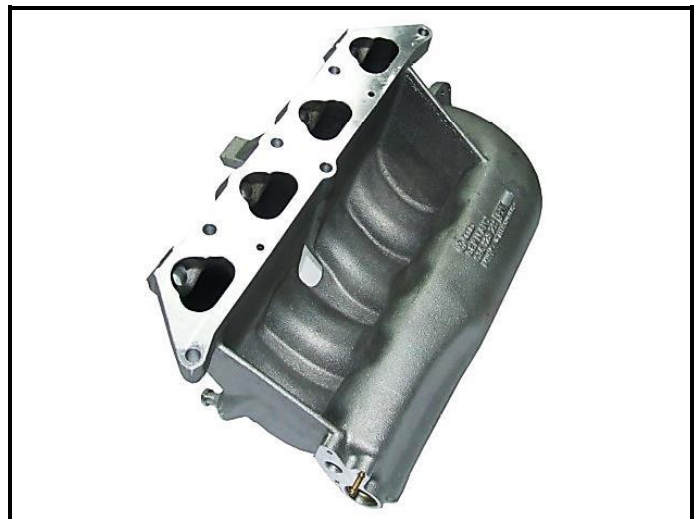
2) INTAKE MANIFOLD – ¾ View BOTTOM
