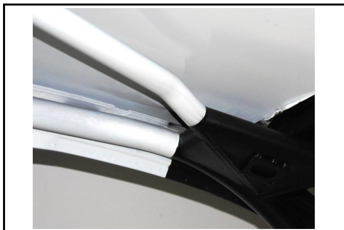
SC-24) Roof reinforcement – bend for helmet clearance
