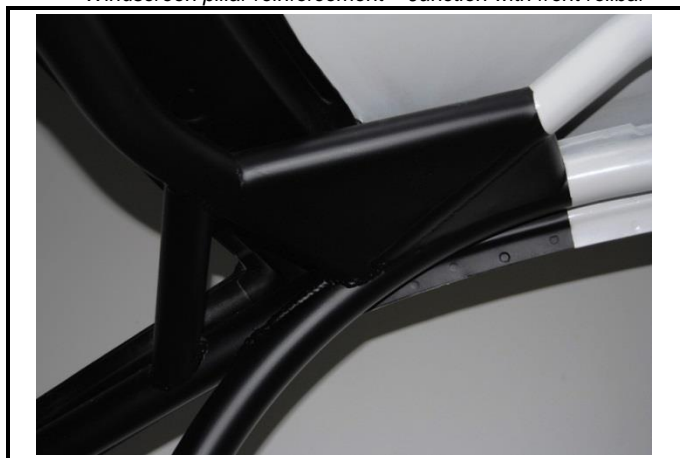
SC-10) Connexion-Renfort montant pare-brise / arceau avant Windscreen pillar reinforcement- Junction with doorbar
