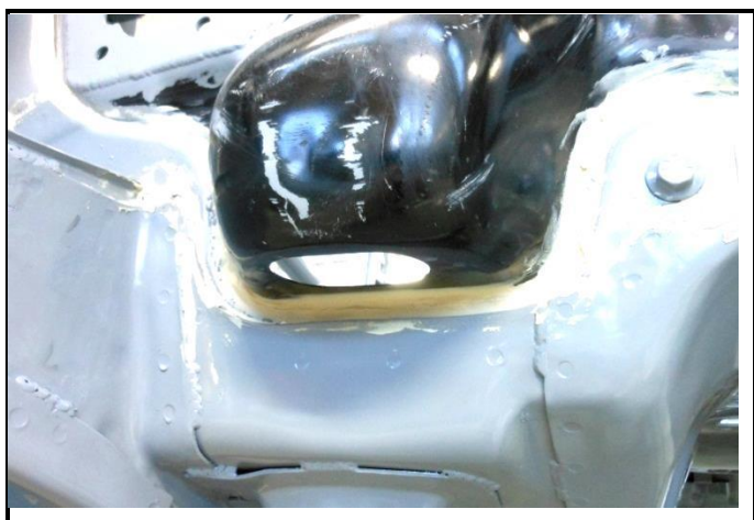
12. Opening in Firewall for Steer Collumn
