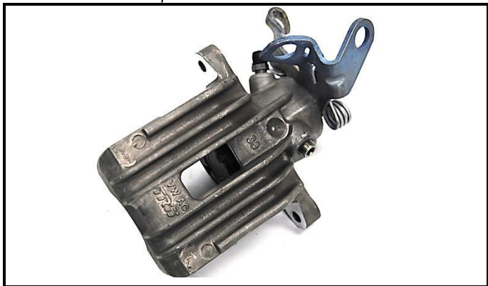
K4-5) Support d'étrier de frein arrière Rear brake caliper support
