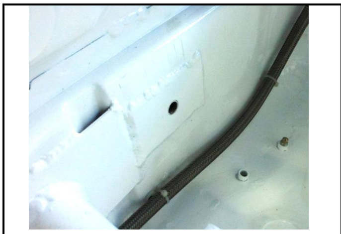
6. Seat Belt Anchor , RH SIDE - DRIVER
