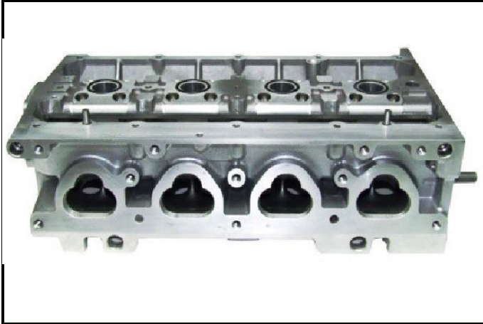
C8-5) Culasse nue vue côté distribution Bare cylinderhead seen from timing side
