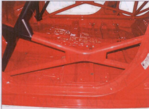
PHOTO 10 DRIVER'S DOOR ANTI-INTRUSION DOORBAR
