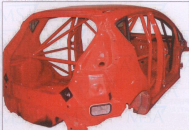
PHOTO 4 MAIN ROLLBAR TO FLOOR ATTACHMENT
