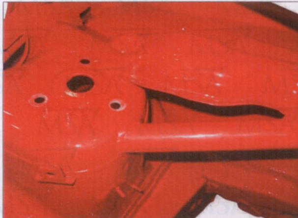
PHOTO 9 ATTACHMENT TO FRONT SUSPENSION
