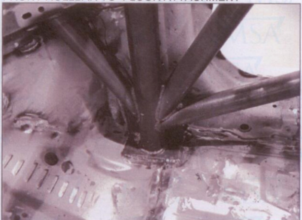
PHOTO 6 FRONT ROLLBAR TO FLOOR ATTACHMENT
