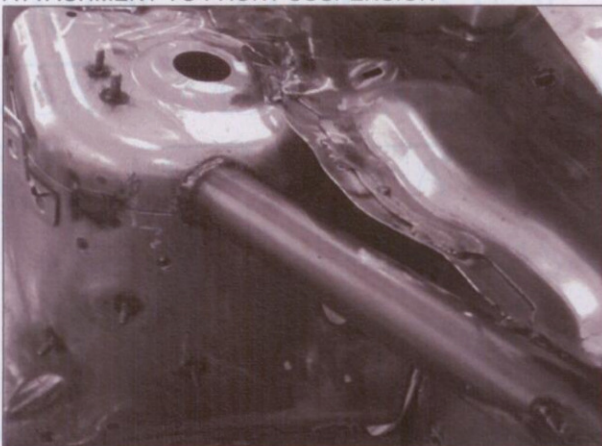
PHOTO 9 ATTACHMENT TO FRONT SUSPENSION
