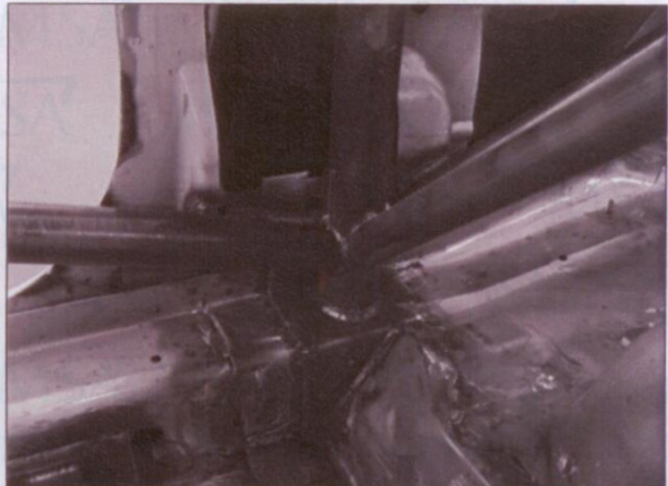
PHOTO 6 FRONT ROLLBAR TO FLOOR ATTACHMENT
