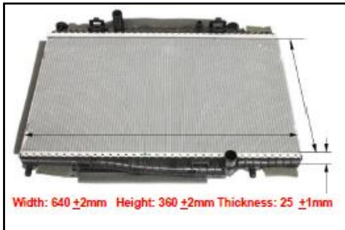
PHOTO 1: 331 Radiator type 4(ZA), dismantled.
