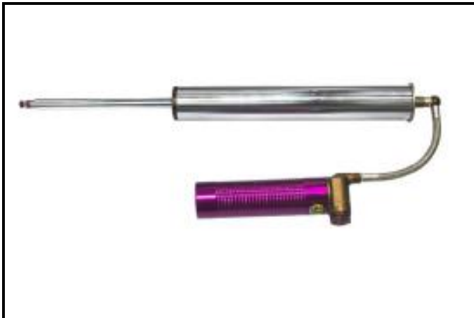
PHOTO 1: 707, Front damper type 4.
