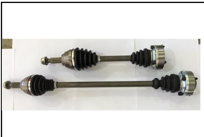
PHOTO 1: 606, Drive shafts, type 2.
