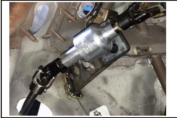
PHOTO 3: 804 cd, Steering multiplier, mounted.
