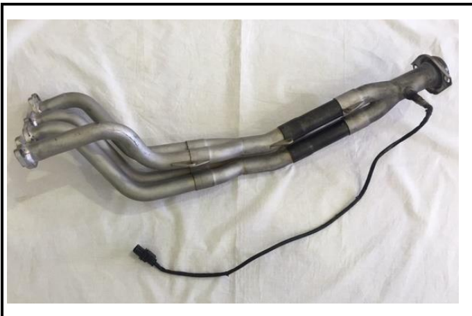
PHOTO 1: 328, Exhaust manifold, type 3.
