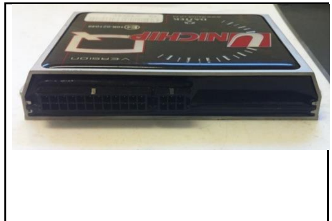
Photo 2: Unichip piggyback ECU connector.
