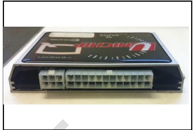
Photo 4: I-driver piggyback assist connector.
