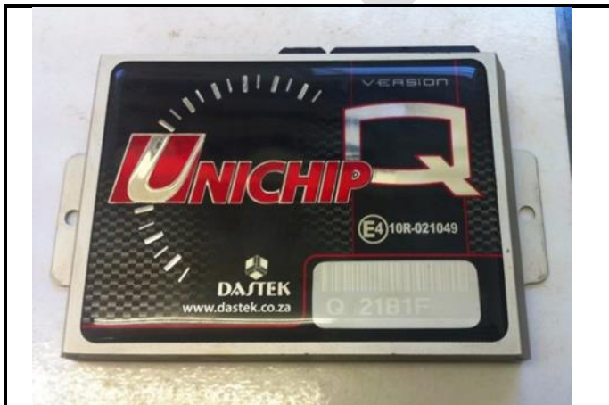
Photo 1: Unichip piggyback ECU.
