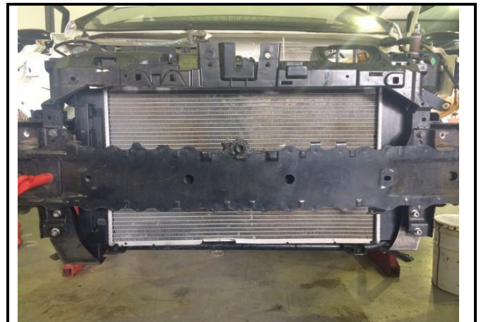
Photo 2: Radiator, type 3(ZA), mounted.
