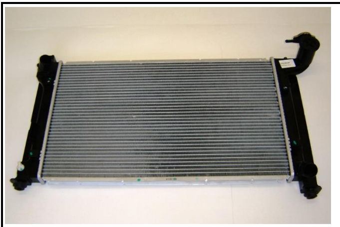
Photo 1: Radiator, type 3(ZA), dismantled.
