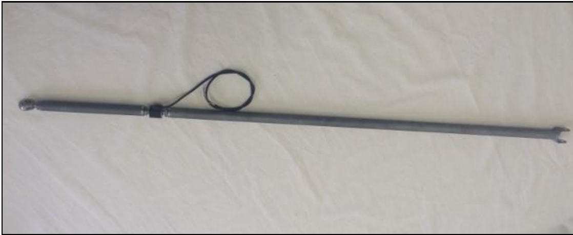
Photo 3: Gear linkage with gearcut load cell, type 2(ZA).
