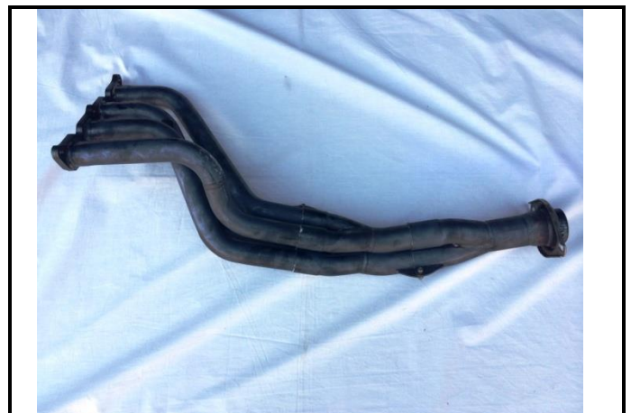
2) Exhaust manifold type 2, photo 2
