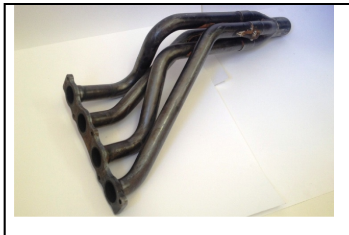
17 Exhaust manifold 4 into 1, type 2
