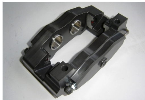
J4-6) Support d'étrier de frein avant Front brake caliper support
