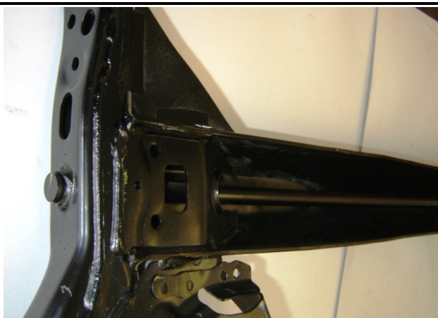
TOYOTA ETIOS PRODUCTION STABILISER AS A UNIT WITH RR SUSPENSION BEAM
