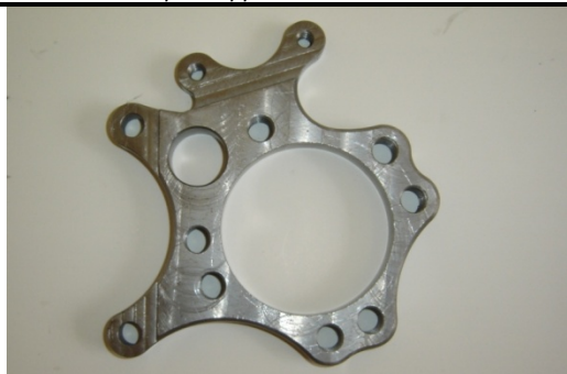
K4-5) Support d'étrier de frein arrière Rear brake caliper support
