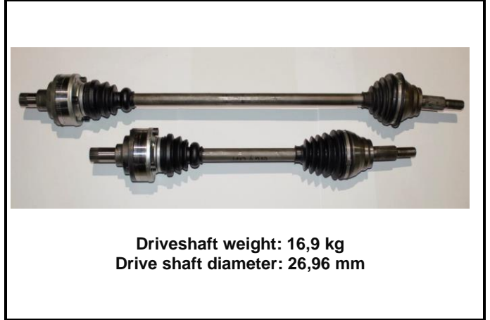
Photo 4: 606-c,d Driveshafts type 3, with tripods replaced by CV joints.
