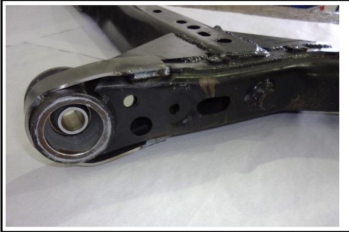
Photo 3: 700-a1, Rear axle type 2, rubber mounting bush replaced with spherical bearing.
