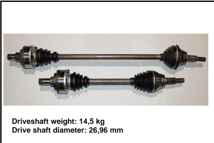
Photo 5: 606-c,d Driveshafts type 3, with tripods replaced by CV joints.
