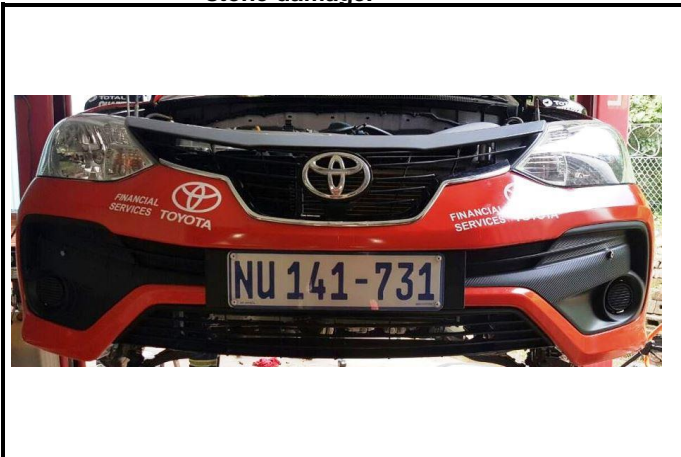
Photo 11: 101 Front bumper bottom bar cut to limit stone damage.
