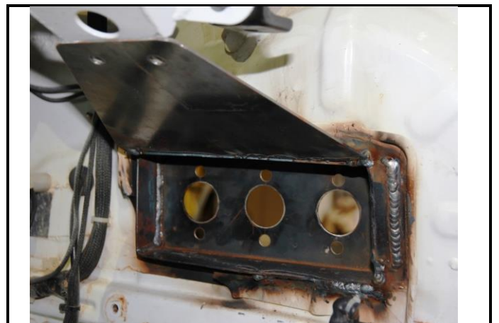
Photo 6. Firewall mount box, rear.
