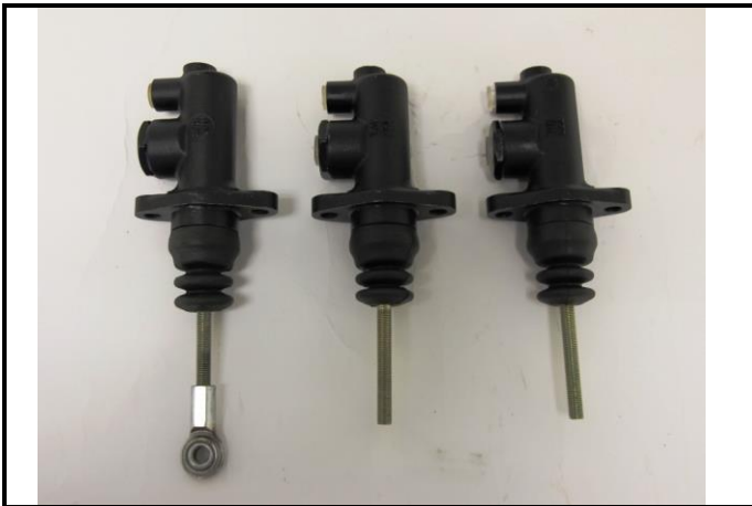
Photo 9. J6-1) Brake & clutch master cylinders, dismantled.
