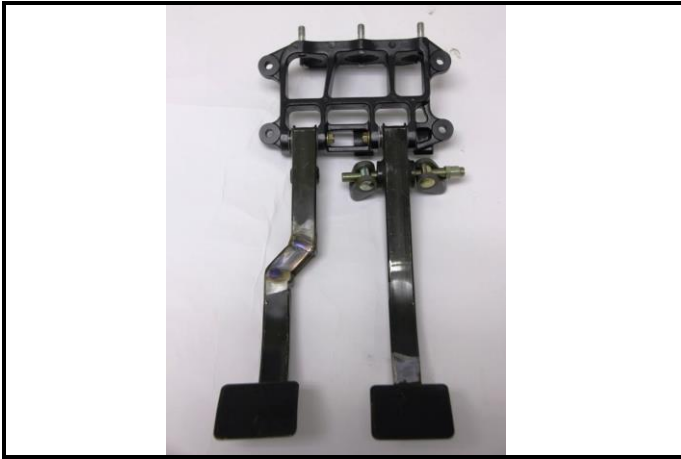
Photo 1. L2-1) Brake pedal box, dismantled, front view.
