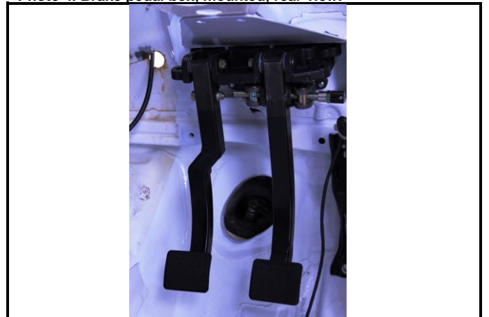
Photo 4. Brake pedal box, mounted, rear view.
