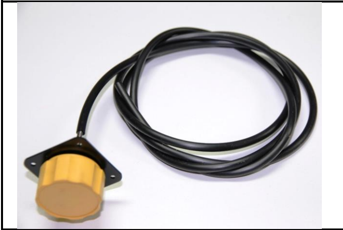
Photo 7. Brake bias cable, dismantled.
