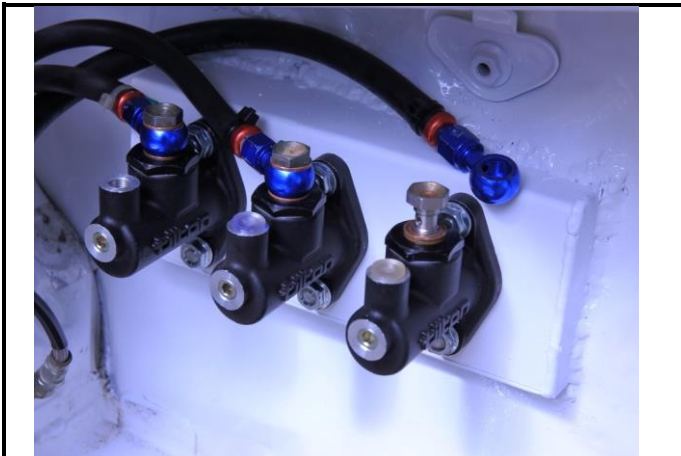
Photo 3. Brake pedal box, mounted, front view.
