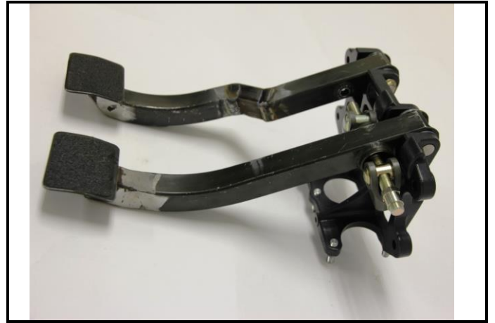
Photo 2. L2-2) Brake pedal box, dismantled, side view.
