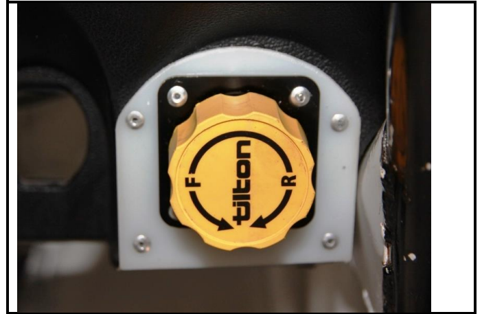
Photo 8. Brake bias cable, mounted.
