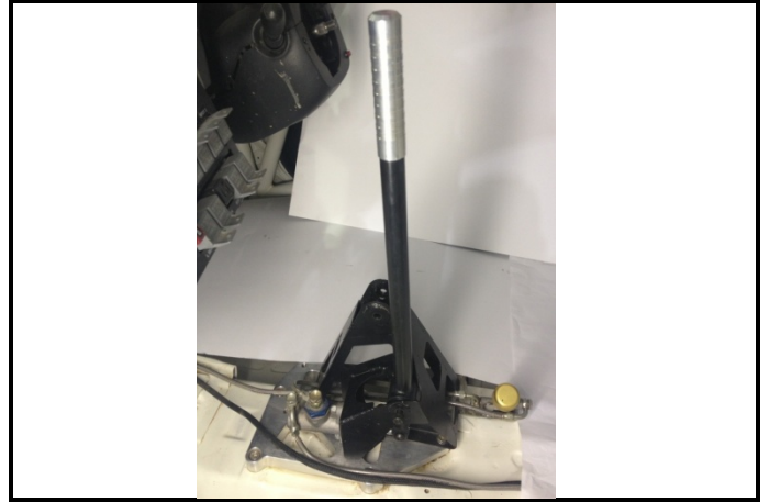
4) Hand brake assy, type 2 - mounted
