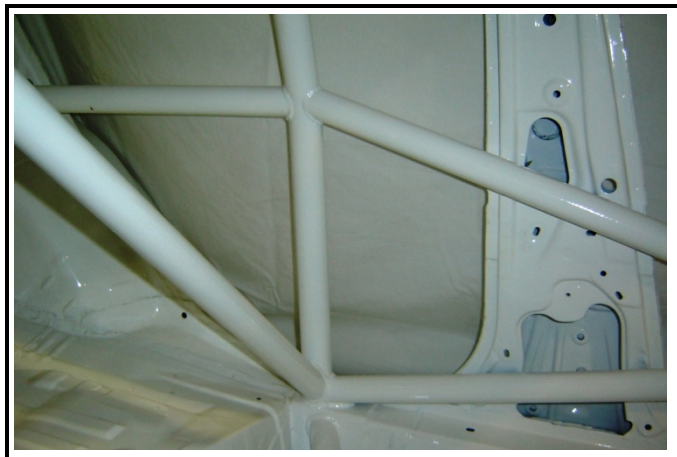
SC-24) Roof reinforcement – bend for helmet clearance
