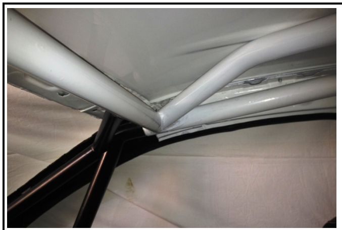
SC-24) Roof reinforcement – bend for helmet clearance
