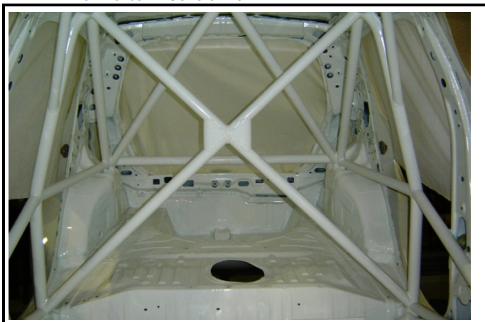
SC-11) Arceau principal – Vue d'ensemble Main rollbar – General view
