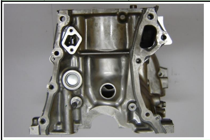
C3-5) Bloc-cylindre nu vu côté distribution Bare cylinder block seen from timing side
