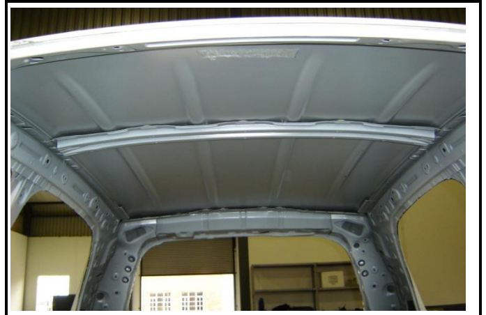
N1-6) Châssis nu – Toit vu de l'habitacle Bare chassis – Roof seen from cockpit
